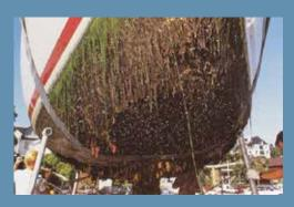
In tropical areas, hull fouling - the attaching of barnacles, weed, slime, algae, etc to the hulls of ships - can increase fuel consumption by 7% after one month and 44% after half a year if antifouling paint is not used.
