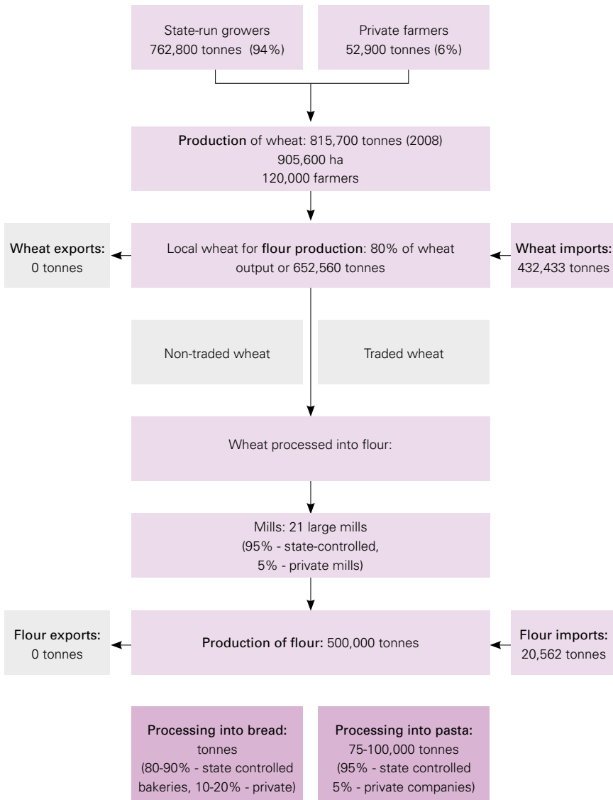
Figure 3.7. Schematic description of the wheat-to-bread supply chain
