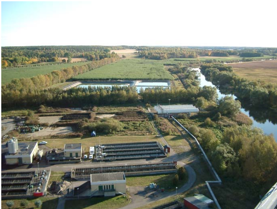
Overview of Enköping sewage treatment works with storage lagoons in the middle ground and willow plantation in the background centre and left.
