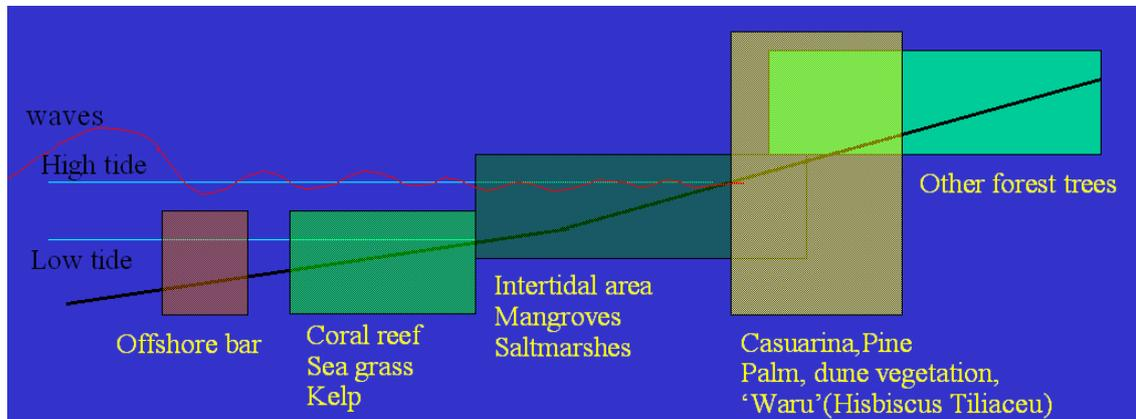
Figure 4.8 The natural protective features of coastal systems
