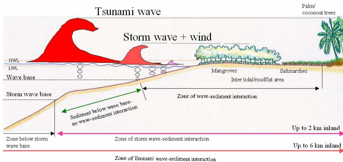
**Figure 4.5 Intertidal/muddy coast (modified from ARC [2000] and French [2001])**
