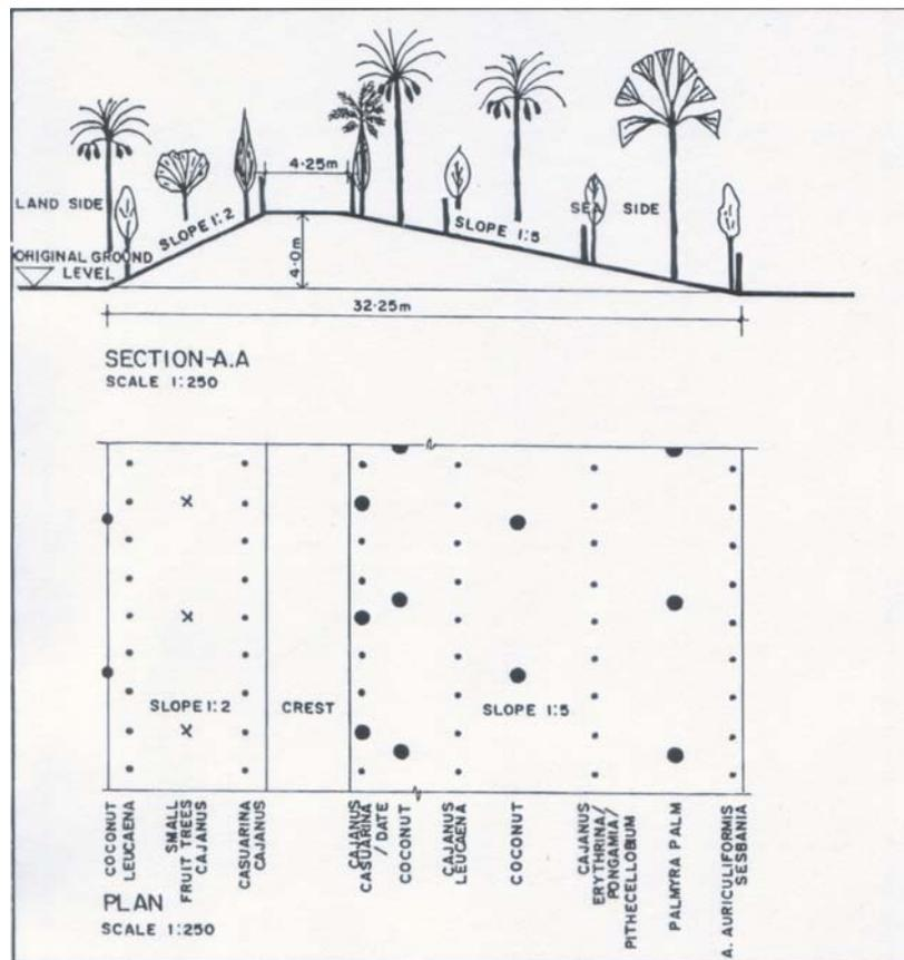
**Figure 4.11 The natural protective functions of coastal forest and trees, starting with water-edge vegetation on intertidal deltas, rising to hydric species on higher soils or land. The green belt model below with coastal embankments (in Bangladesh) combines different type of trees, including fruit trees, which benefit local communities (Clark, 1995)**
