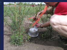
Measuring N 2 O and CO 2 fluxes using non-steady state vented chambers.
