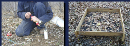
Employing suction lysimeters and litter traps to measure nutrient cycling within SRWC plantations.
