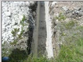
Figure 2. Solvay wastebeds consist of fairly uniform material. This trench is about 3m below a layer of soil and gravel cap that has been installed to create parking space.
