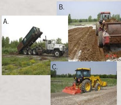
Figure 5. Delivery (A), applications (B) and incorporation (C) of brewery biosolids to the Solvay wastebeds
