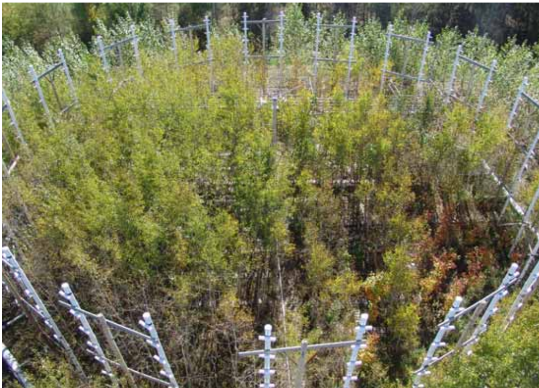
Figure 7.12. A typical 30-m wide FACE treatment ring with 5 aspen clones (left ½) and mixed aspen/maple (lower right) and mixed aspen/birch (above right). Photo credit: D.F. Karnosky.
