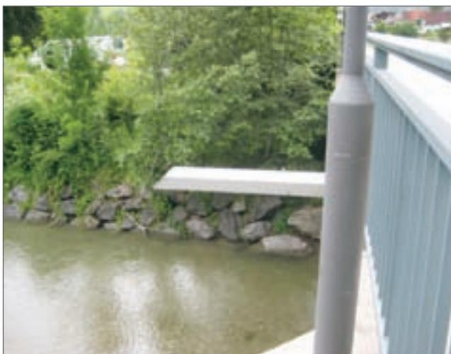
Fig.1 Variants of radar gauge installation
