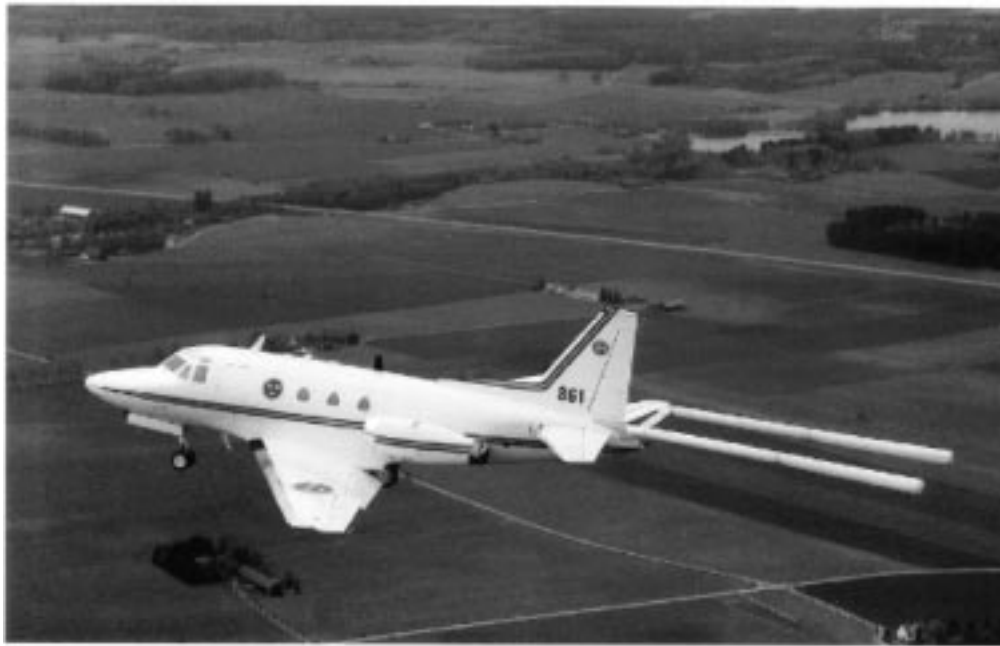
Fig. 1. The Sabreliner aircraft with the CARABAS antenna system deployed (courtesy of FMV:Prov).
