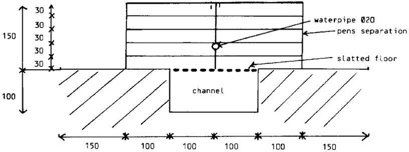
**Figure 10.5. Dimensions of feed trough for cattle (in cm).**
