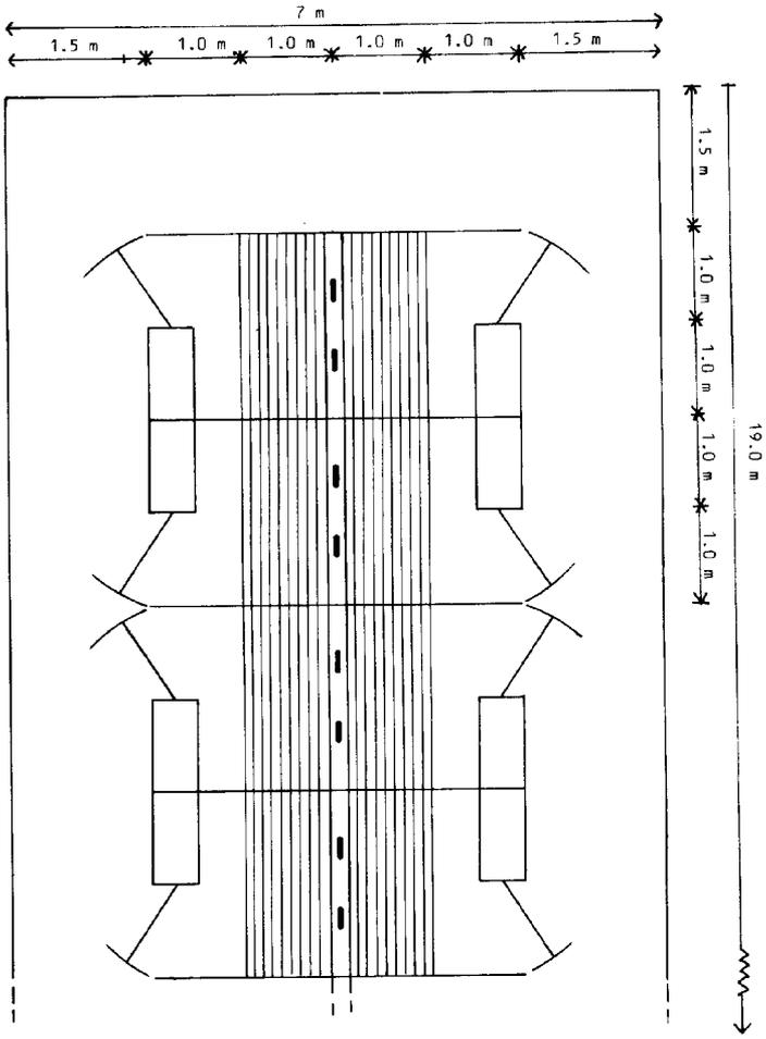
Figure 10.3. Dimensions of cattle slats (in mm).
