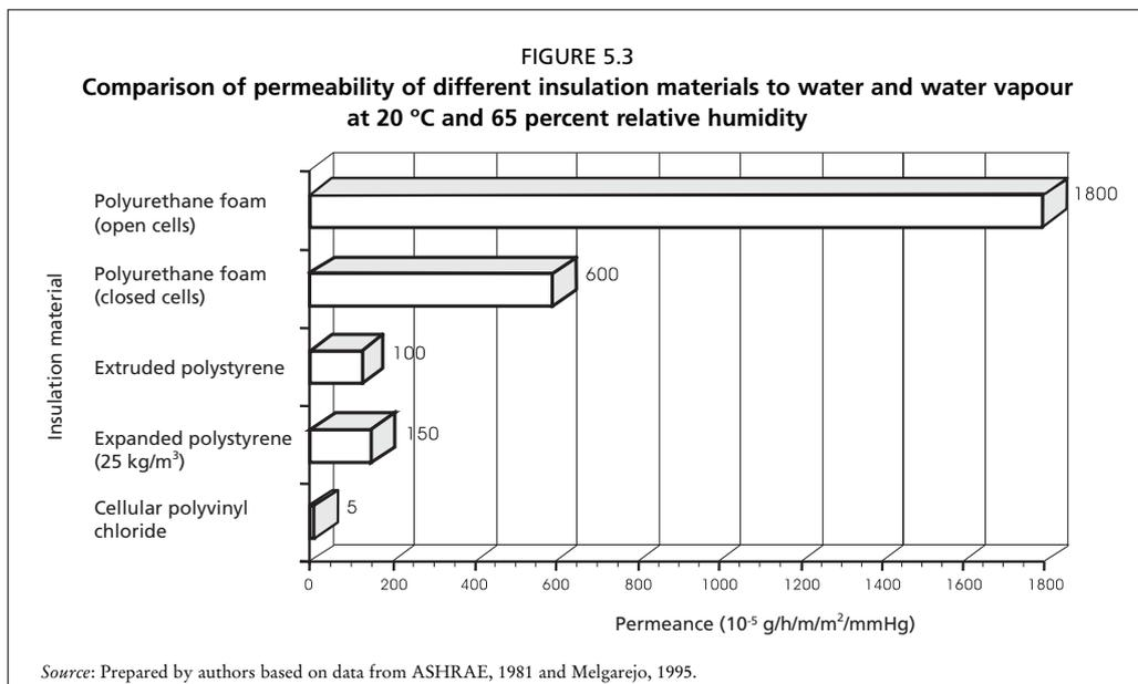
expanded polystyrene. Their main technical limitation is the fact that they are more likely to absorb water than expanded polystyrene, and can burn and produce toxic substances during ignition. Figure 5.3 shows the permeability of different insulation materials to water and water vapour.
