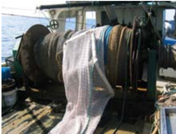
Figure 5: The use of a selective grid on Mediterranean trawler needs in particular the possibility of storing it on the net drums (Sardà et al. ; communication No. 8).
