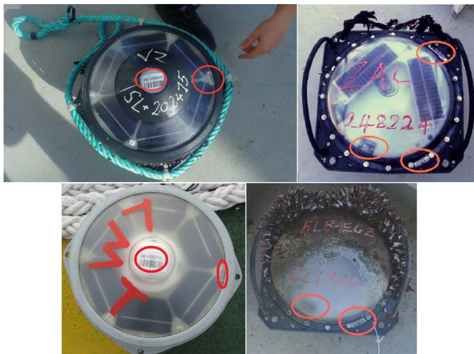
Figure 1. Examples of brands of satellite buoys used by purse seine fishers to track the geospatial position of dFADs. The locations of buoy manufacturer unique identification codes are identified with red ovals. White and red codes painted on the buoy surface are identification codes added by owners. Bottom-right: a used buoy with biofouling. Bottom-left and top: new buoys (bottom left image courtesy of Beau Bigler, Marshall Islands Marine Resources Authority; other images courtesy of Mikel Basterretxea, AZTI Tecnalia)
