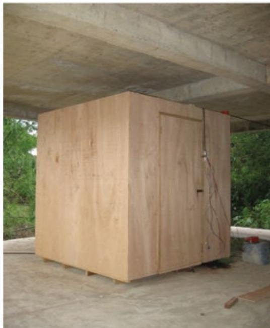
*The PHTRC Storage/cooling chamber equipped with an evaporative cooling pad with charcoal as the wetted media. A submersible pump is used to move water from a sump tank to a water distributor at the top of the cooling pad.*
