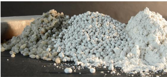
Figure 1: Polyhalite can be processed into chips, granules or powder
