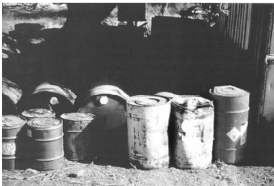
FIGURE 2 Abandoned pesticide containers (barrels) blown close to disintegration by the high pressure of obsolete pesticides kept in them for years
