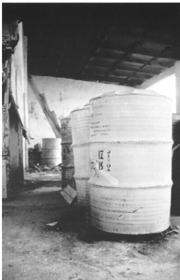
FIGURE 6 Distended barrels that have leaked liquid pesticides into the ground since the bottoms have cracked open through rust and sheer chemical pressure
