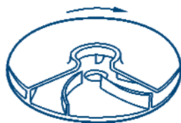
Centrifugal Impeller. Shroud partly cut away showing vanes.
