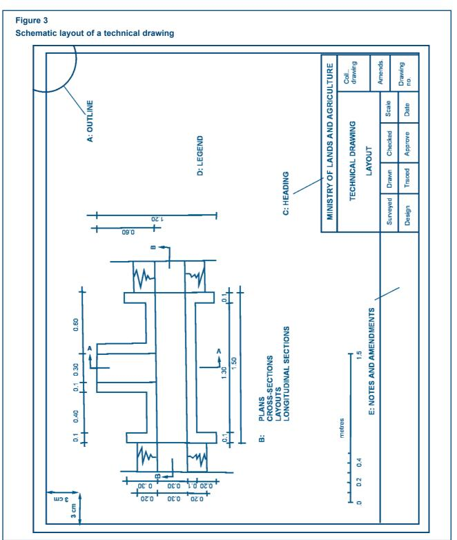
Figure 3 gives a schematic layout of a technical drawing. The details (A, B, C and D) will be explained in the next sections,
