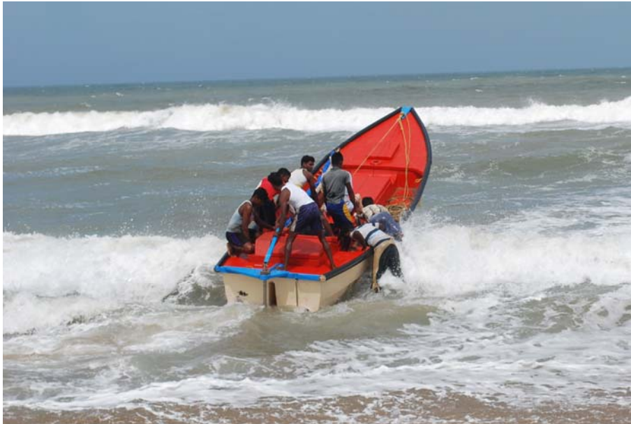
Figure 25. New design of FRP Boat introduced in Tamil Nadu, India (Photo: BOBP-IGO)
