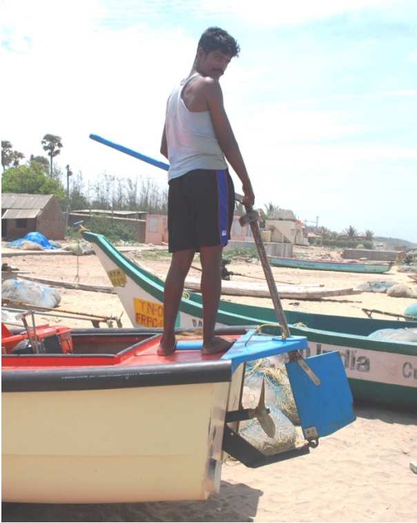
Figure 27. Liftable propulsion system, the BOB-drive.
