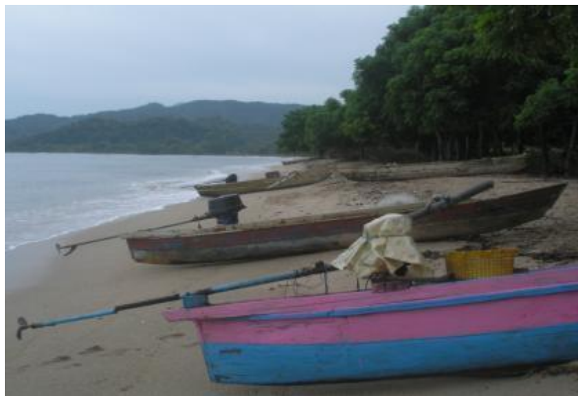
Figure 3-37. Wooden boat with (outboard) motor attached, known as "ketinting" boat
