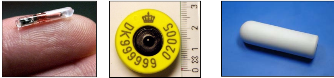
Figure 7: Examples of electronic devices - From left to right: injected chip, ear tag and ruminal bolus
