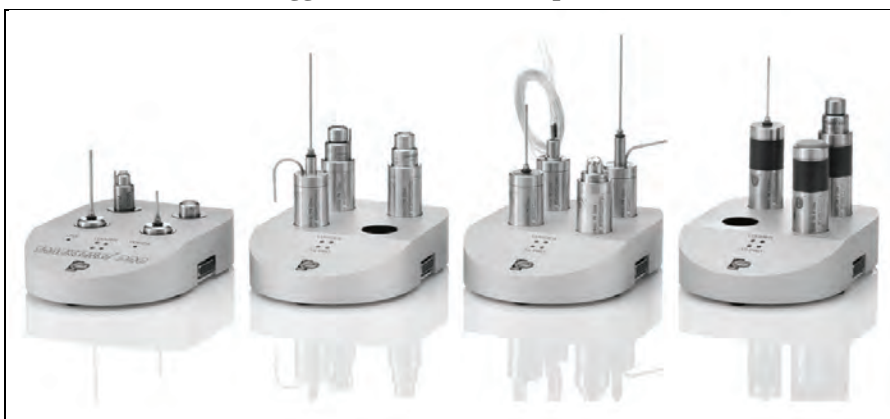
Picture 1. ELLAB dataloggers used for thermal process evaluation
