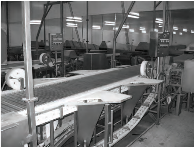
Picture 4. Modern Cabinplant line for preparation and packing of mackerel
