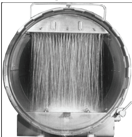
Picture 7. Flow pattern inside a Steriflow cascading retort
