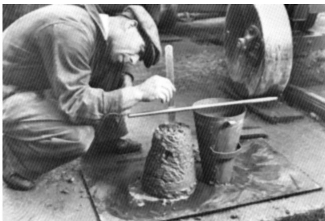
PLATE 8.1 The slump test
