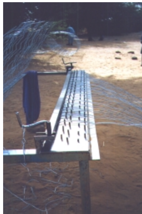
PLATE A3.3 Pairs of wires disposed on the loom
