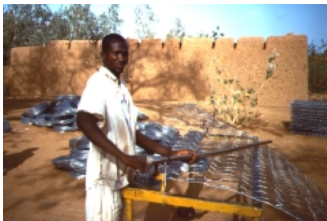
PLATE A3.5 Completed mesh removed from the loom
