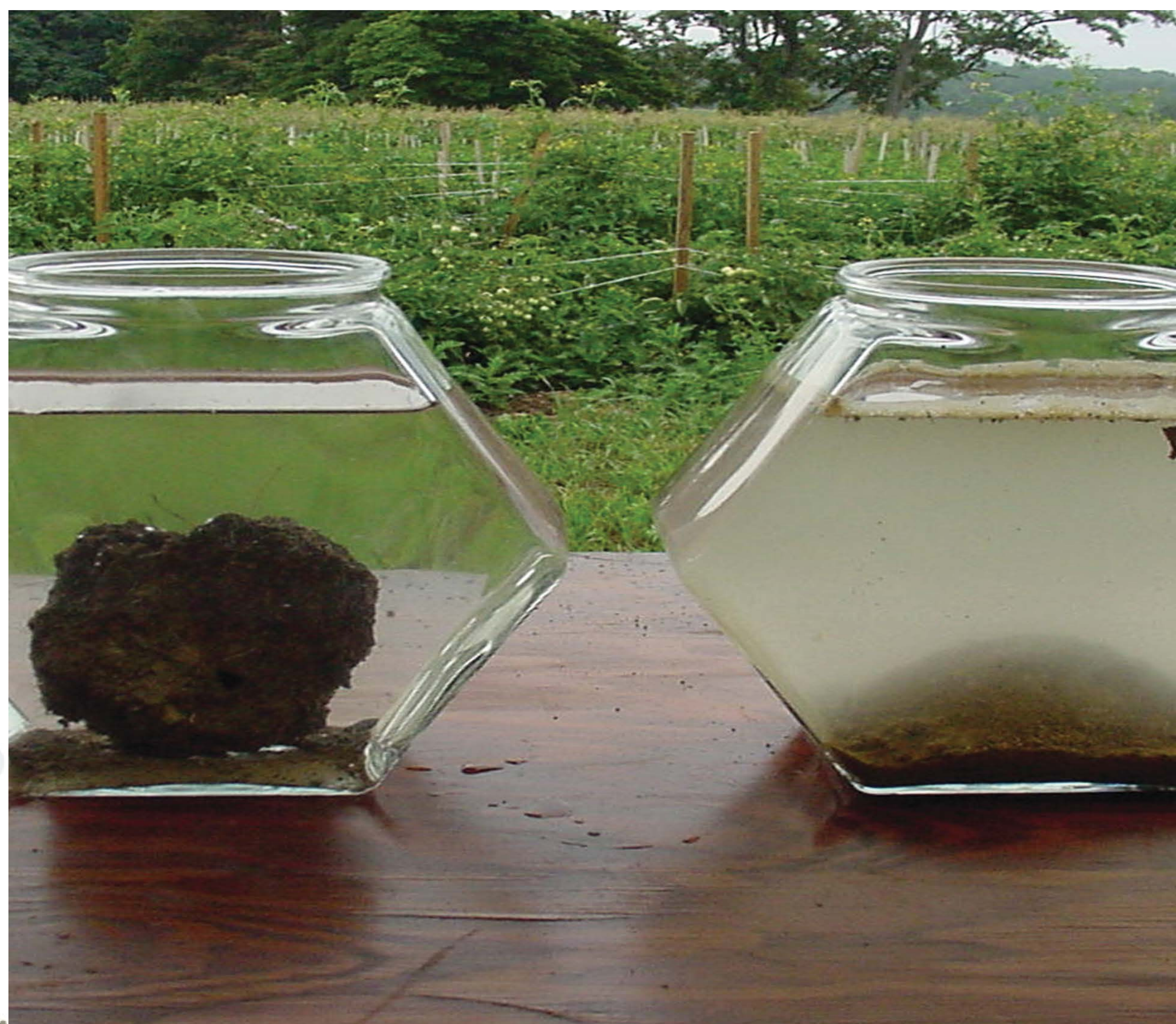
Fig. 2: The same soil under different management systems. The soil on the left has more SOC, is more stable, absorbs and holds more water and nutrients: It has sequestered 57.500 Kgs per hectare of CO 2 in that time ©Rodale Institute
