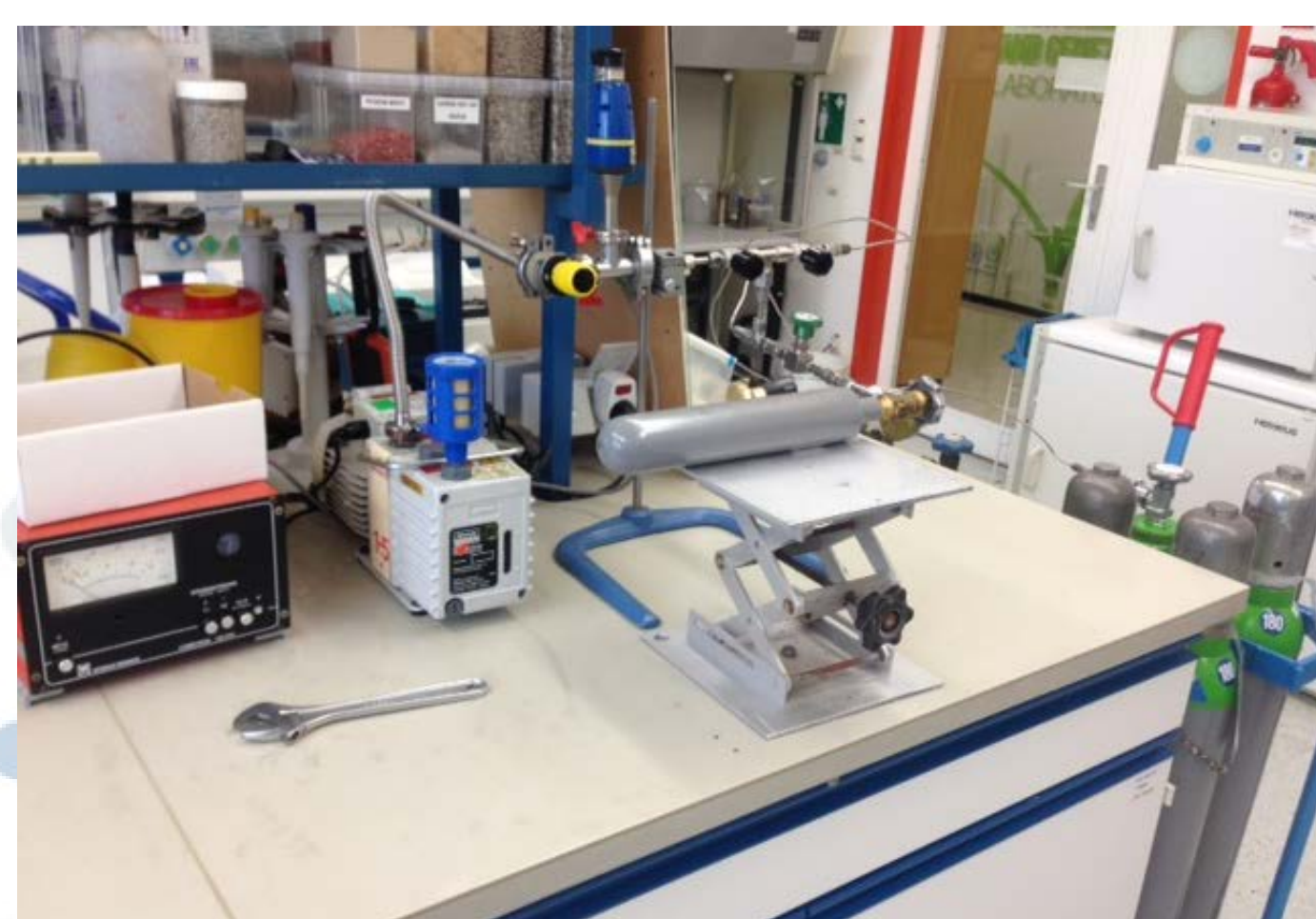
Fig. 1: Gas mixing line linked to a vacuum pump, pressure gauge, \text{CO}_2 and synthetic air gas tanks to make reference gases for laser stable isotope analyzers
