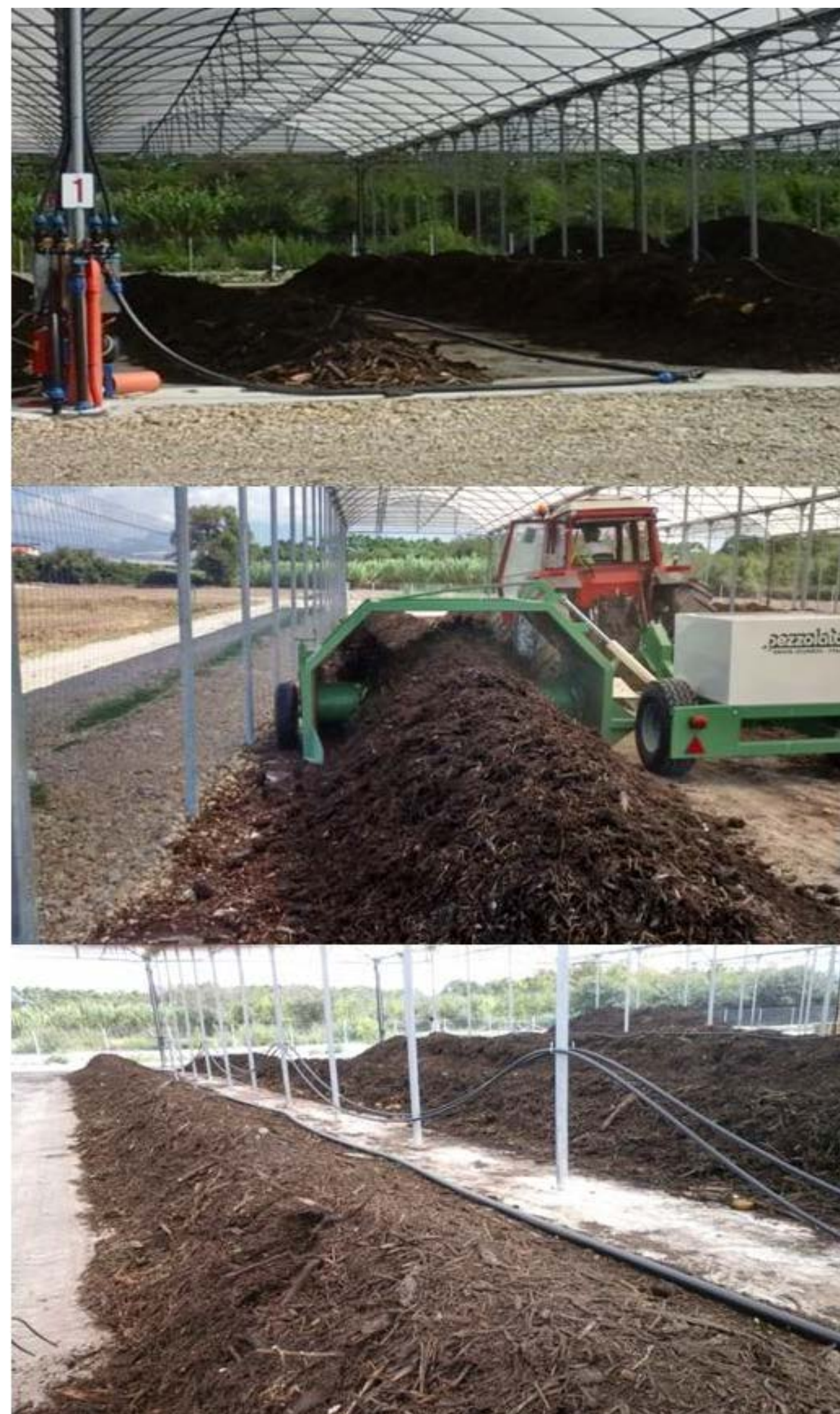
Fig. 1: On farm composting facility attained in CarbOnFarm project- 4000 m 2 -12 composting lines -2000/4000 tons green compost year -1
