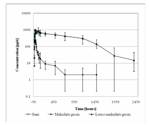
Figure 4a: Concentration changes of malachite green and leucomalachite green during and after bath exposure to 0.032 mg/L of malachite green.
