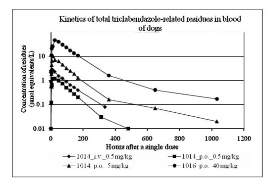
Figure 8: Kinetics of total radioactive residue in blood of dogs dosed with [<sup>14</sup>C]-triclabendazole
