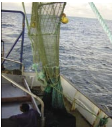
Shrimp trawl with sorting grid (expanded view). Shrimp and fish that pass backwards in the trawl are guided by a funnel to the bottom of the backwards slanting metal grid. Shrimp and fish of comparable size will pass through the slots of the grid and go to the codend, while larger fish and other organisms (e.g. jellyfish) will slide upwards over the grid and are released through the outlet.
