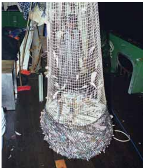
The last section of this square-mesh codend is replaced with diamond-mesh to prevent shrimp escape.
