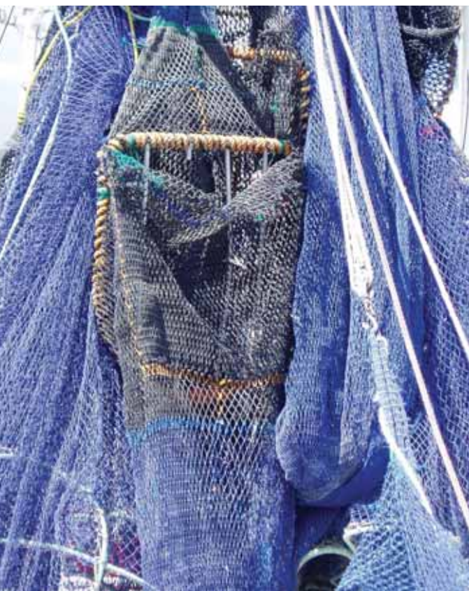
The broken bar of this TED may allow turtles and other large animals to enter the codend and be caught. Alternatively these animals may become jammed in the grid.
