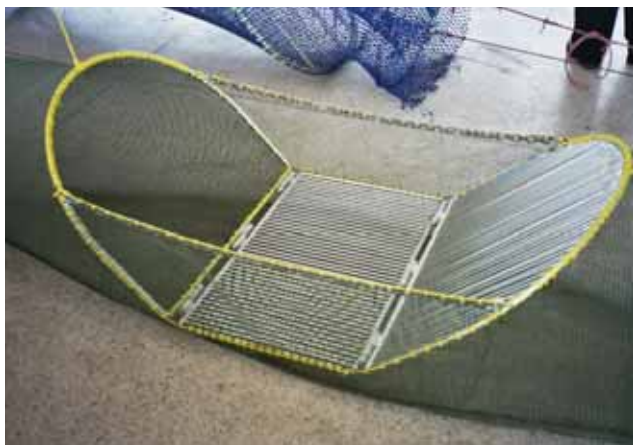
The JTED is a BRD that filters small fish including trash fish from the catch but not the larger shrimp.
