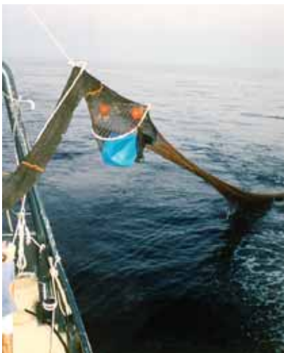
A tombstone-shaped grid is a compromise between a rectangular - and an oval-shaped grids. The canvas sheet in front of the grid is used to assist the rapid exclusion of animals from the trawl.
