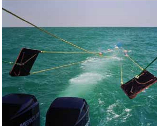
The use of long sweeps and headline floats will increase the amount of bycatch that enters a trawl.
