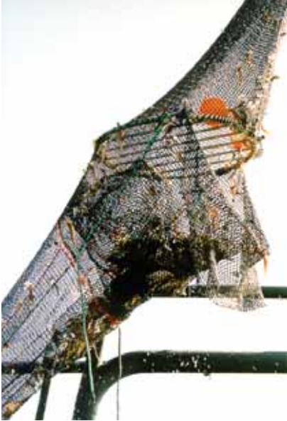
Oval grids conform well to the cylindrical shape of the codend. Note the escape opening extends part way round the sides of the grid.
