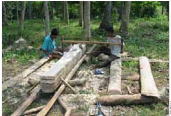
Two-person handsaw is used for primary breakdown of logs in the forest
