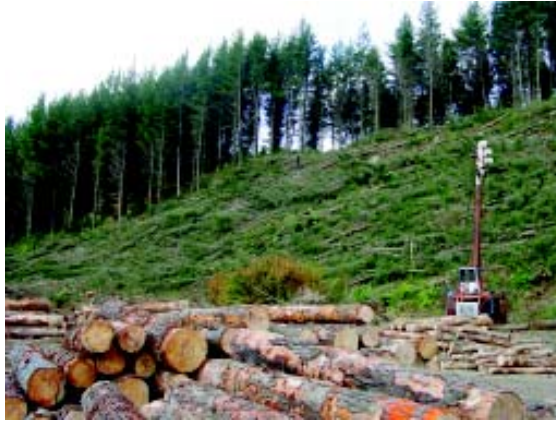
A cable hauler in Lake Taupo Forest harvesting mature trees with a piece size of 2 to 3 tonnes (courtesy Lake Taupo Forest Trust).
