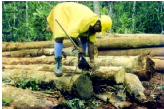
Log scaling using calipers at Nakavu forest (courtesy SPC/GTZ Pacific-German Regional Forestry Project).
