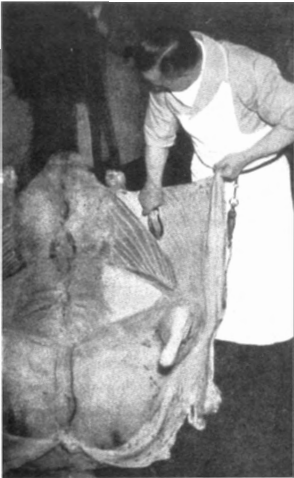
Figure 16. The flaying machine in operation. It is driven by compressed air and has the same action as a hand-knife, the blades being kept flat against the hide, with a backward and forward motion.
