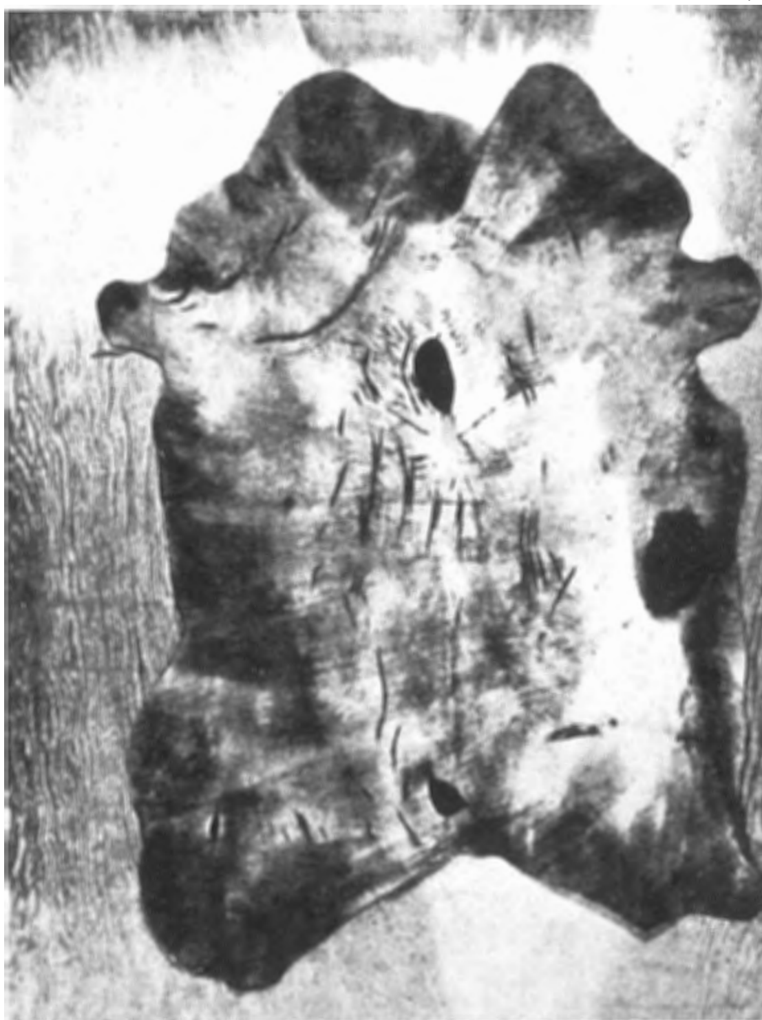
Figure 64. Leather made from a calf-skin which has been badly cut and damaged by knives, so that its value is considerably reduced. (Courtesy of Department of Information, Nairobi, Kenya.)
