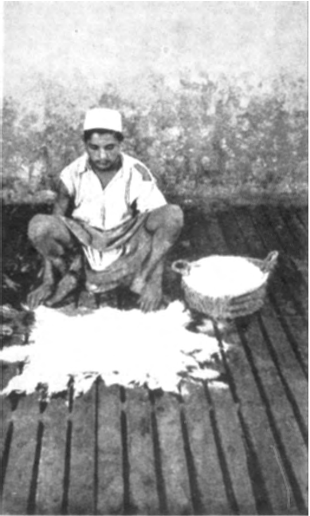
Figure 51. After washing and shaking off the excess water, the first skin is laid on wooden slats to allow for free drainage, and half its weight of good common commercial salt is spread over the entire skin.
