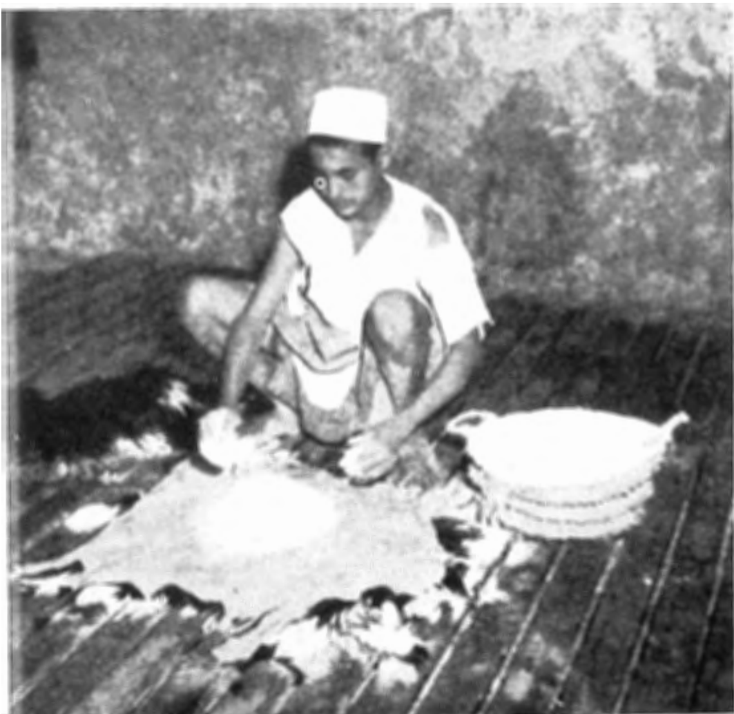
Figure 52. Another skin is spread on the top and this also has half its weight of salt spread on it.
