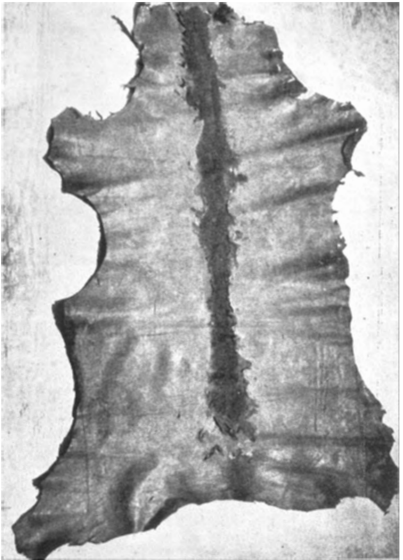
Figure 47. Local putrefaction damage along the backbone line, which is worse on the grain side than on the flesh side. The part of this pole-dried hide covering the pole has putrefied during drying because there was no air circulation along this line. (Courtesy of Department of Information, Nairobi, Kenya.)
