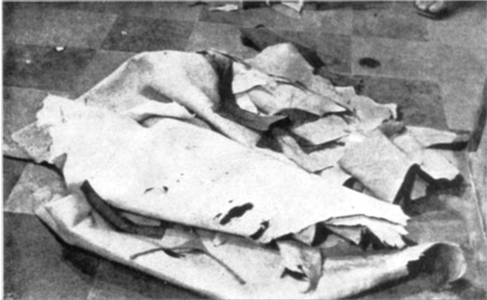
Figure 55. Leather showing a number of putrefaction holes and other defects which mean losses for the leather-goods maker.
