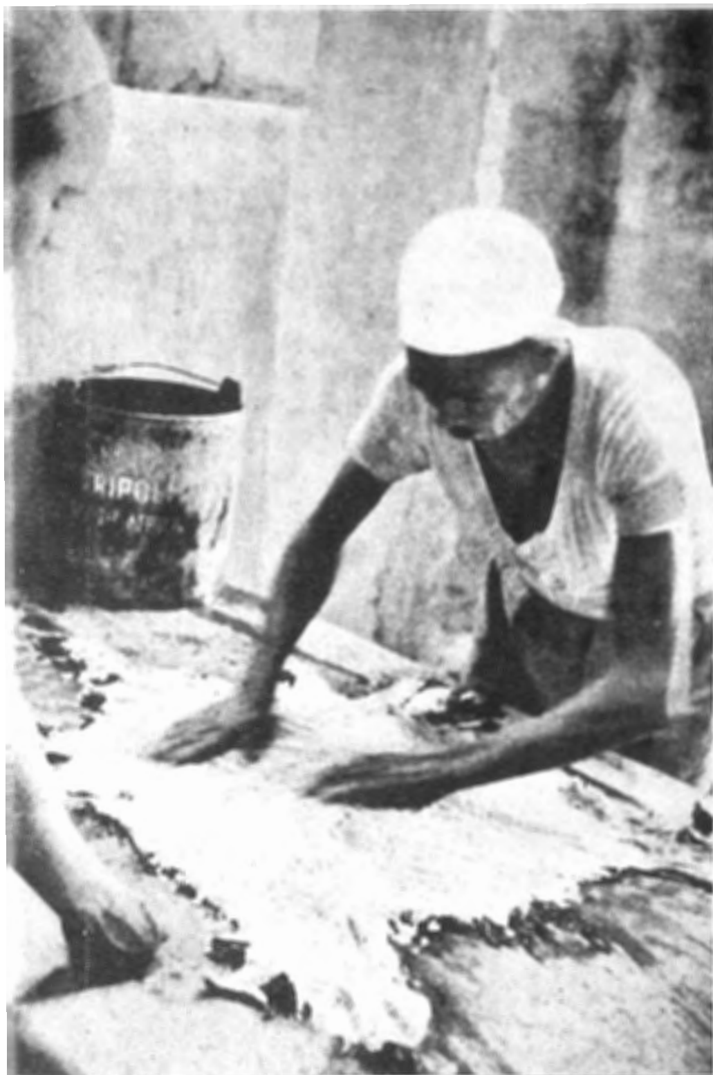
Figure 50. The best way to start “dry” salting is to wash the flesh side of the skin with clean water on a sloping table, as shown here. The hair is not washed, as it would retain too much water.
