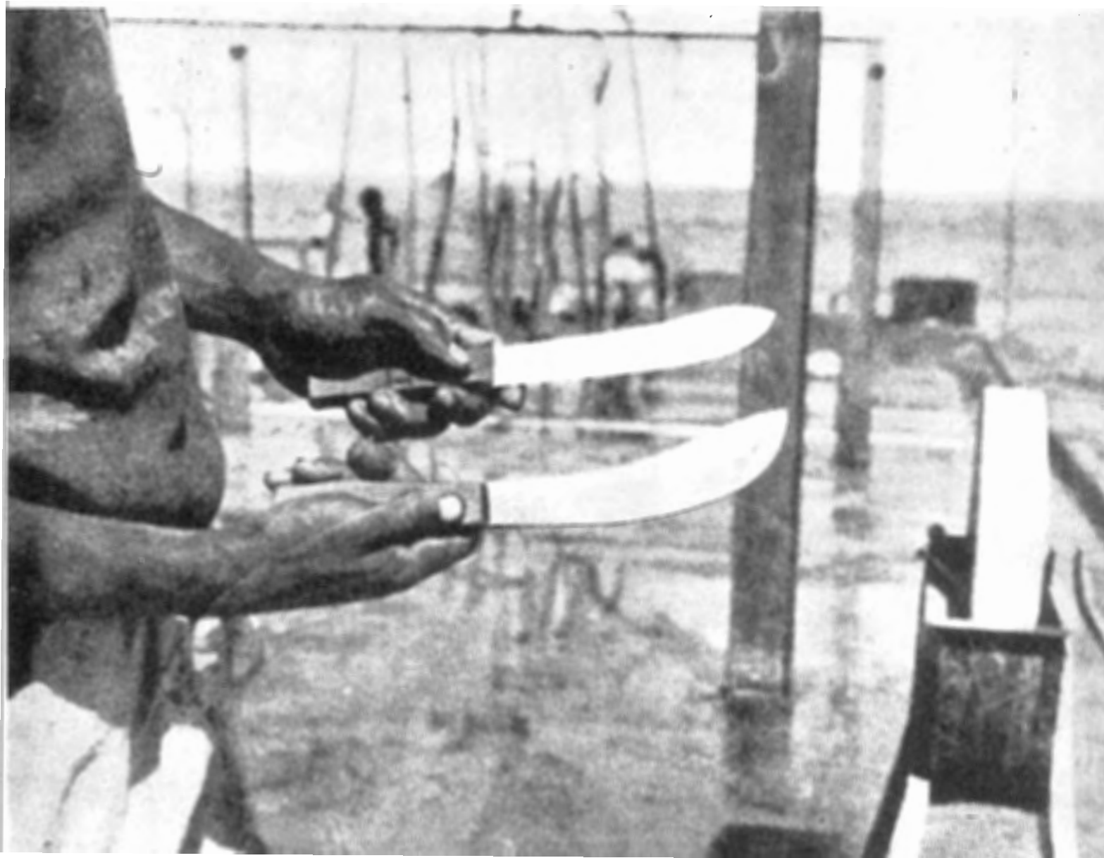
Figure 76. Above is shown a two-edged pointed knife which, having the straighter edge, must only be used for ripping. The knife shown below, being curved, could be used for flaying. The grindstone on the right is essential to maintain a sharp cutting edge.
