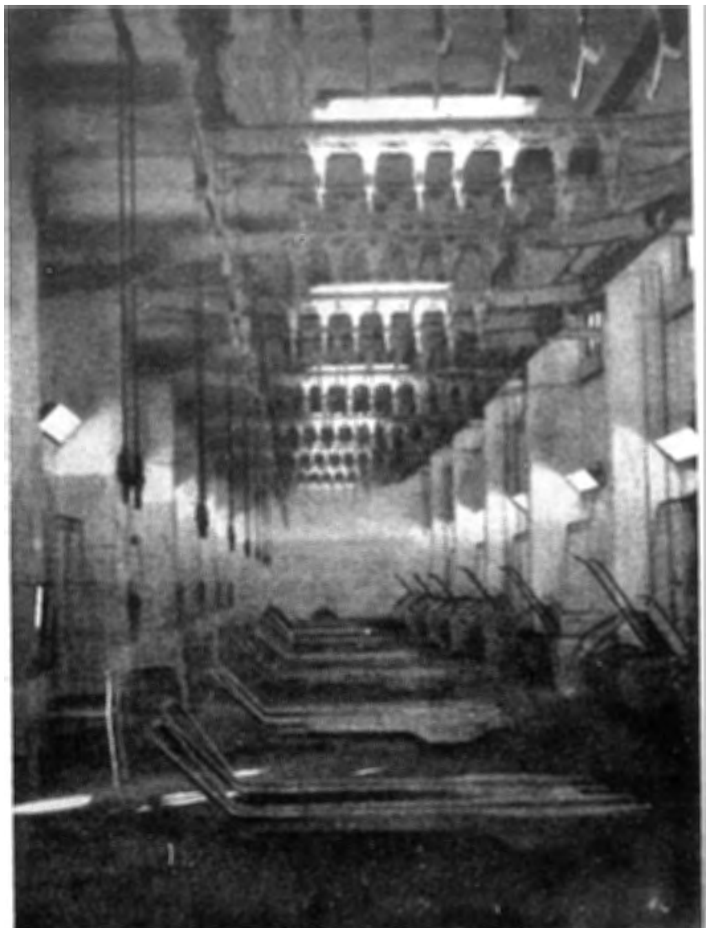
Figure 4. A contrast to flaying methods "in the field." This photograph shows a modern European abattoir equipped with steel flaying cradles, electric hoisting gear, special bins and trucks for handling the entrails and offal, and a conveyor system for handling the carcasses. Note the light and airy design, white tiled walls and clean concrete floor.
