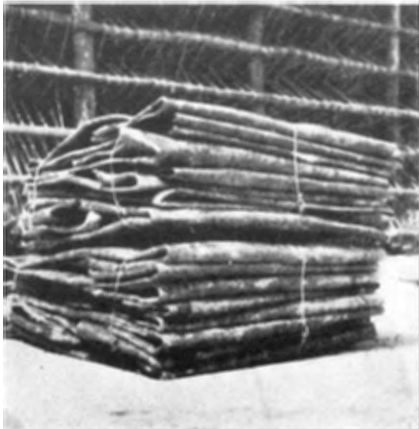
Figure 70. Folded hides, tied together with wire. They will be damaged during transport at the places where wire and hide are touching. It would have been better if a piece of gunny or skin waste had been placed between the hide and the wire as protection.
