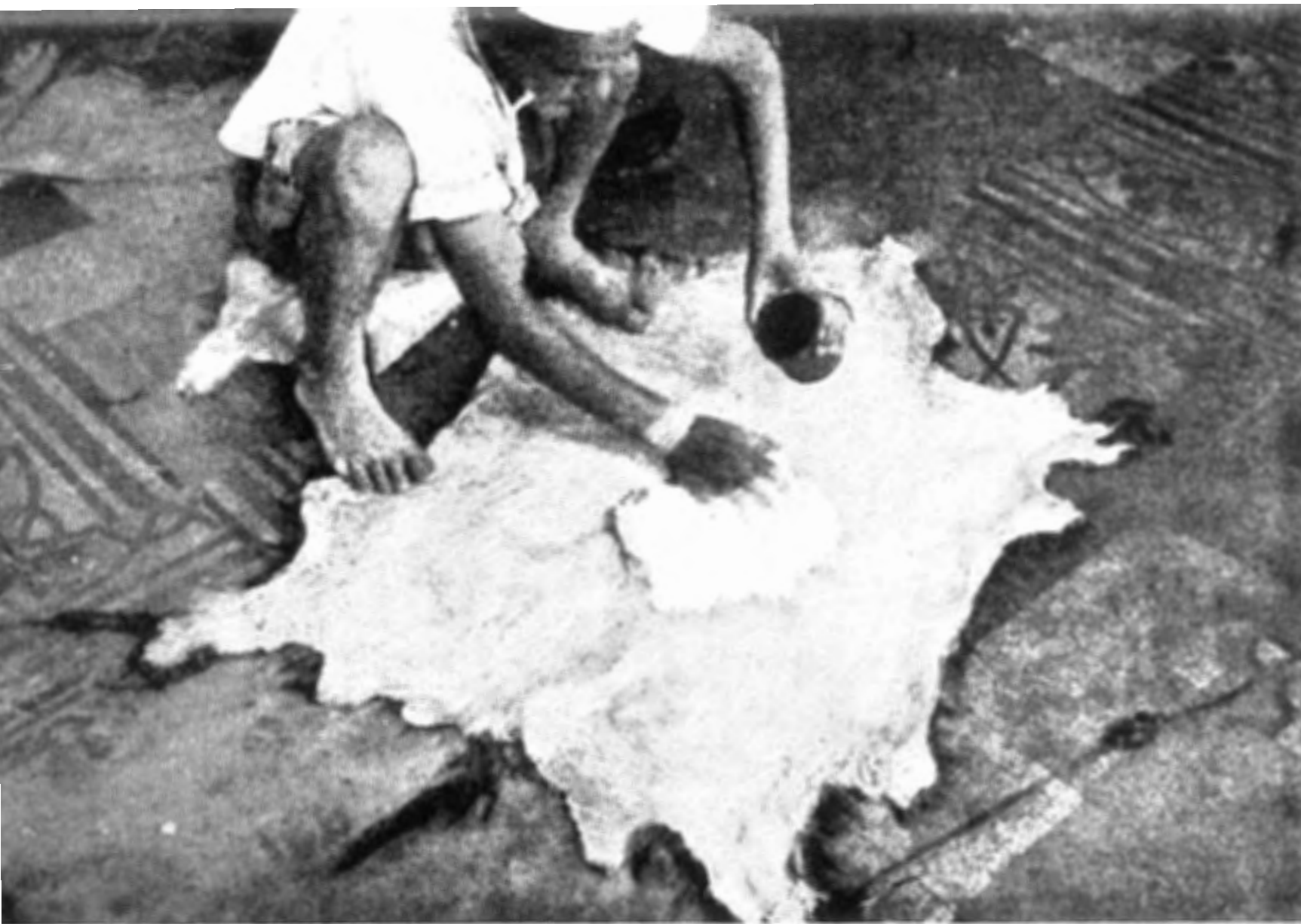
Figure 56. A faulty method of curing goatskins and sheepskins with salt. The wet skin is placed on the floor, a double handful of salt is placed in the middle and a canful of water added, and the salt and water are spread over the flesh.
