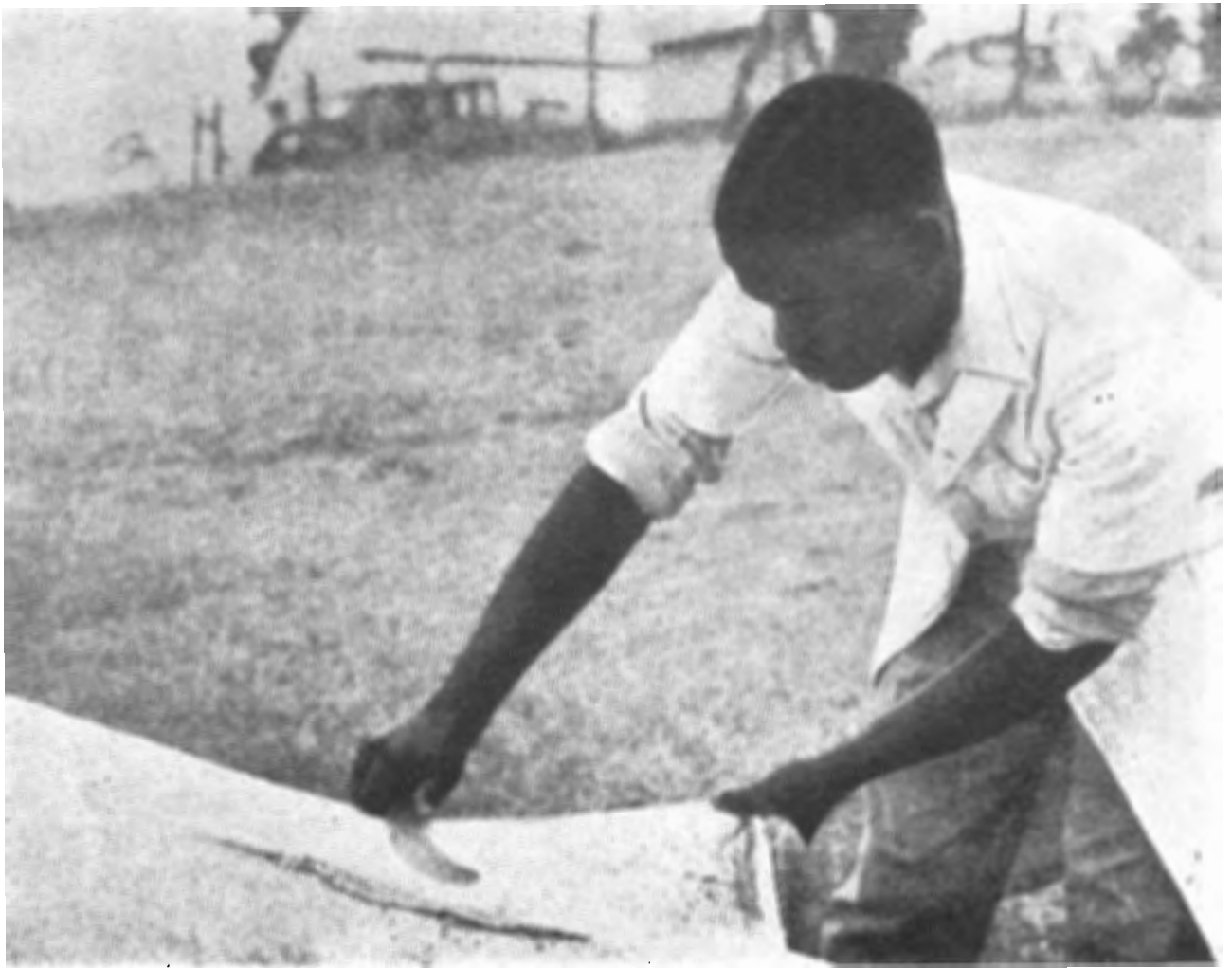
Figure 19. Fleshing on a flat, smooth table. A very sharp curved-edged knife is used. Note the position of the worker's hand and the flaying knife. (Courtesy of Department of Information, Nairobi, Kenya.)
