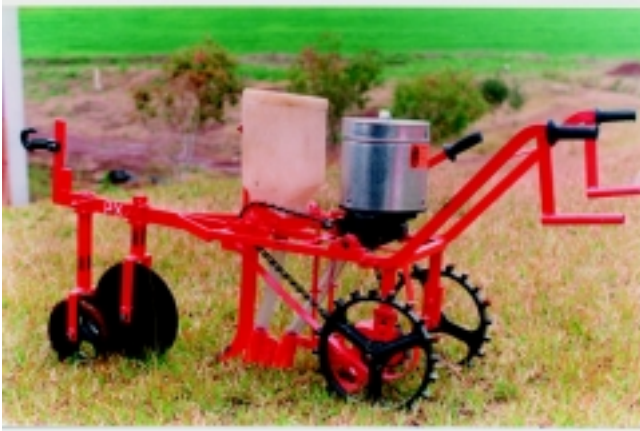
PLATE 68 Direct-sowing equipment for animal production produced in the Itaiópolis municipality
