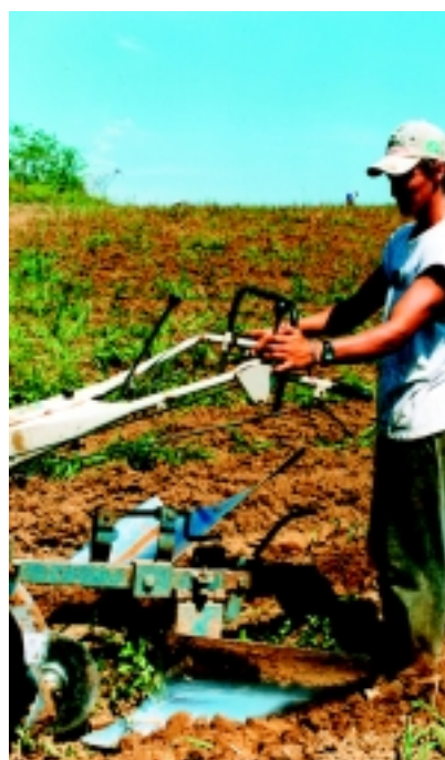
PLATE 25 Micro-tractor with a mouldboard plough for opening furrows in a minimum tillage system
