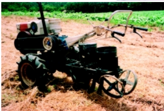
PLATE 54 Modern equipment produced in Atalanta municipality, with the fertilizer and seed hoppers in a longitudinal position
