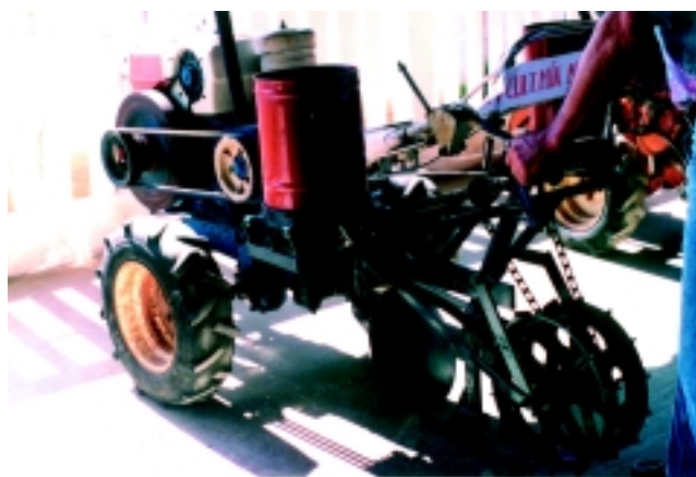
PLATE 52 Direct-sowing equipment for grain adapted for mini-tractors - an advanced system developed by small agricultural entrepreneurs in the Alto Vale de Itajaí region
