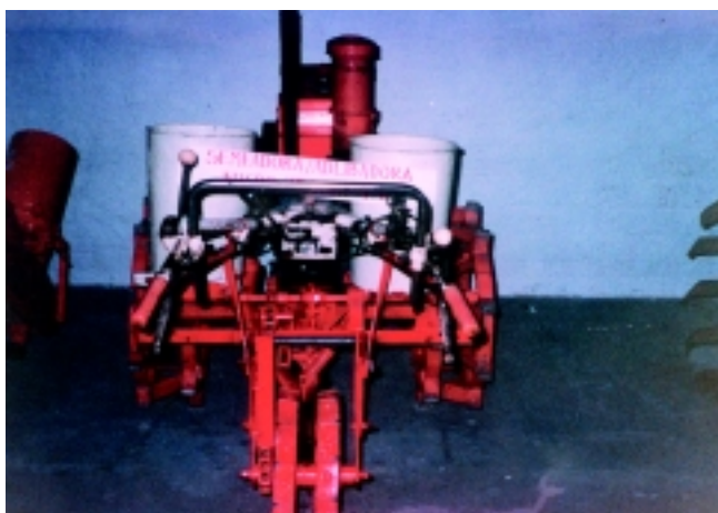
PLATE 53 One of the earlier versions, with fertilizer and seed hoppers made of plastic on mini-tractors with an iron wheel
