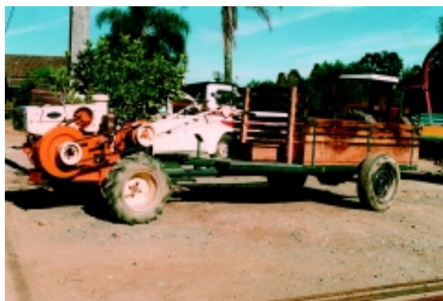
PLATE 56 Cart with traction in the wheels coupled to a mini-tractor, which is capable of operating in steeply sloping areas
