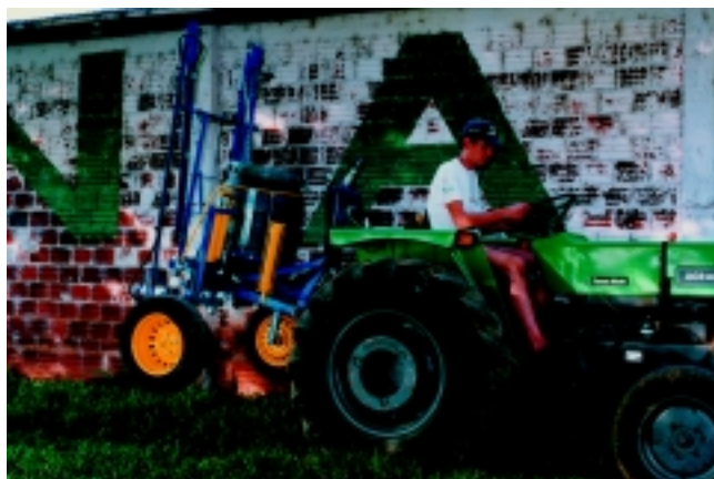
PLATE 92 Sprayer for coupling to tractors with a round tank of 150 litres (with a square tank 250 litres capacity)
