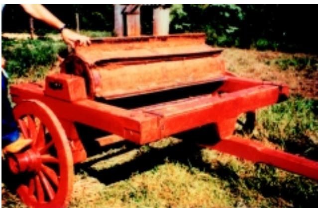
PLATE 76 Roller with blades with a wooden cylinder in the transportation position
