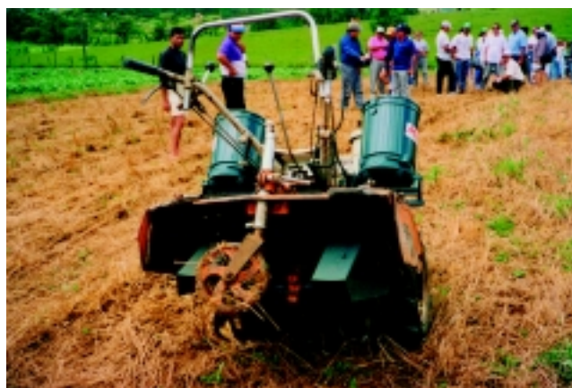
PLATE 51 Mini-tractor adapted to the minimum tillage system for onions. Shows details of the hoppers for seed and fertilizer (which did not exist in the original version), and of the protective cover over the rotary hoe unit to avoid seed and fertilizer being scattered outside the furrow
