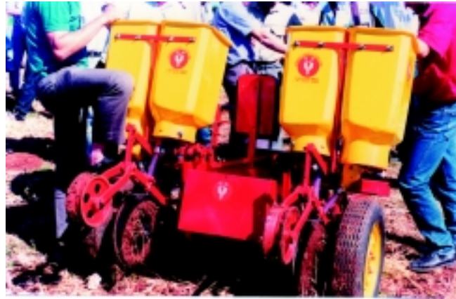
Plate 72 Two-row direct-sowing and fertilizing equipment with tyred wheels from Rio Grande do Sul. View from the rear
