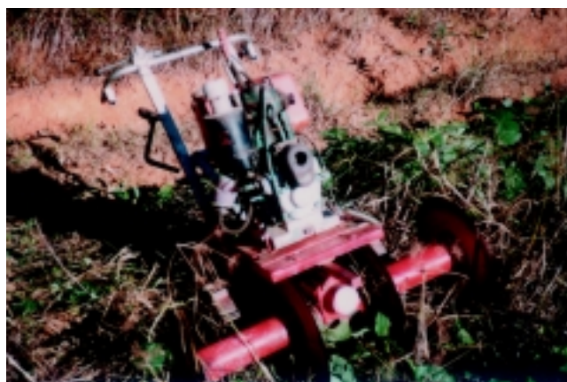
PLATE 81 Mini-tractor developed in the Ibirama municipality to slash mucuna in steeply sloping areas
