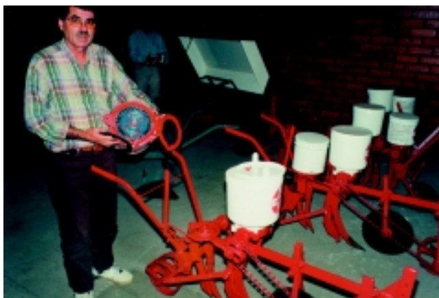
PLATE 65 An entrepreneur showing the most recent version of his direct-sowing equipment for animal traction.
