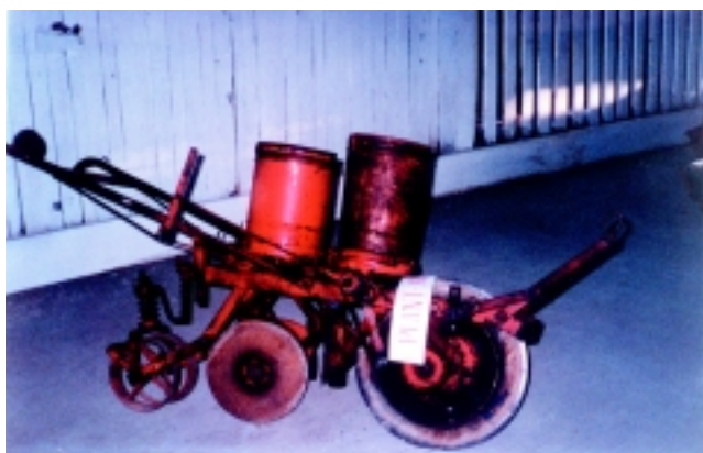
PLATE 60 One of the first versions of direct-sowing equipment for animal traction produced in the region Alto Vale de Itajaí, showing details of the front disc for cutting the residues
