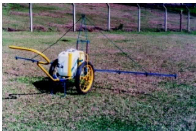
PLATE 88 A model currently in production with various improvements - in the tank (made of plastic, 50 litres), transport system, traction bar and spray bar (with 8 nozzles)
