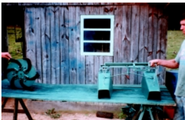
PLATE 59 Details of the rotary hoes and the protective covers over the hoes opening the furrows
