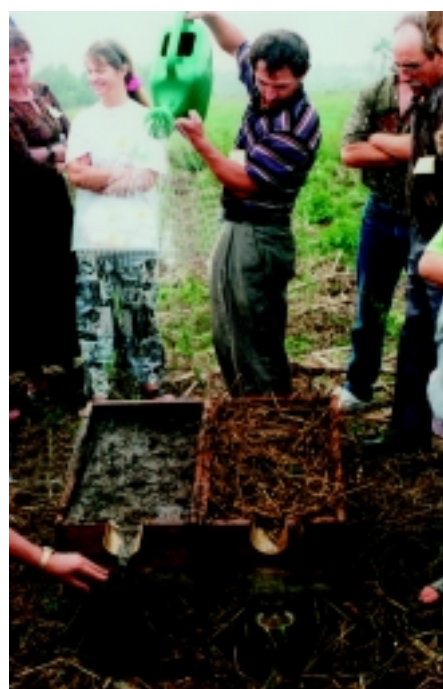
PLATE 5 Effect of the impact of raindrops on bare soil. The breakdown of aggregates is started by the impact of raindrops, and the runoff transports the detached particles.
