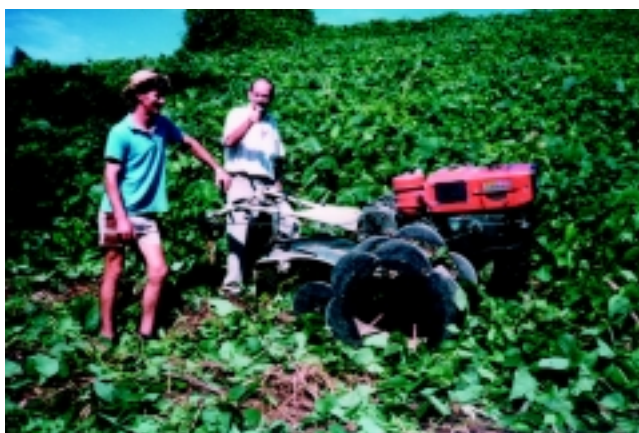
PLATE 82 Mini-tractor with parts of discs welded to the wheels to slash mucuna, Ibirama municipality
