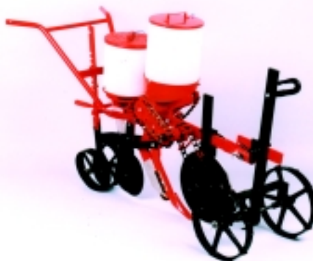
PLATE 66 Latest version of direct-sowing machinery for animal traction produced in Mafra municipality.
