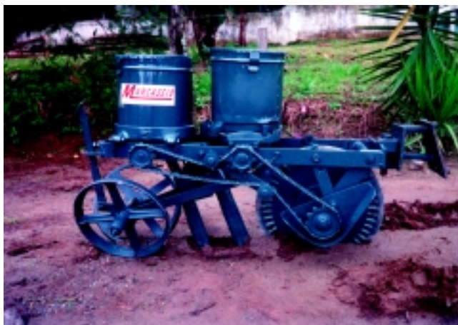
PLATE 54 Modern equipment produced in Atalanta municipality, with the fertilizer and seed hoppers in a longitudinal position
