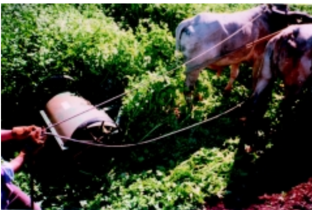
PLATE 77 Roller with blades with an iron cylinder being used to flatten cover crops (forage radishes)
