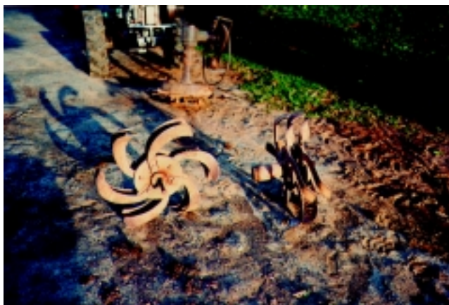
PLATE 50 Example of the first sets of rotary hoes which substituted the conventional hoe assembly
