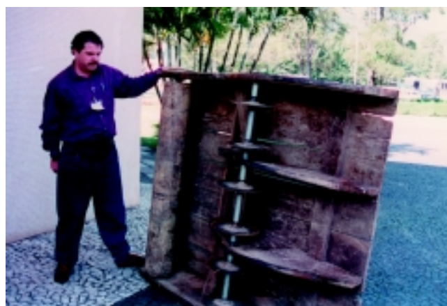
PLATE 80 Roller with discs developed by small farmers in the Alto Vale de Itajaí region
