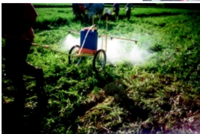
PLATE 87 Operation of a manual sprayer in the Mafra municipality. Contact of the operator with the chemical product during application is practically eliminated
