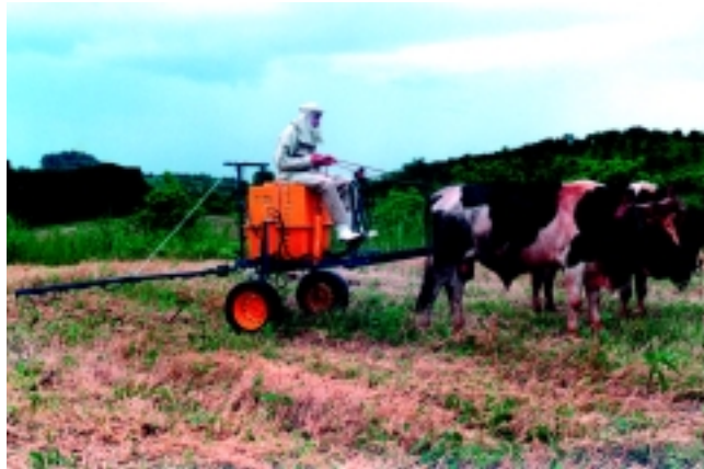
PLATE 90 Model with fibre-glass tank, 250 litres capacity, a spray bar of seven metres and 14 nozzles, wagon wheels for transport, and operator seat
