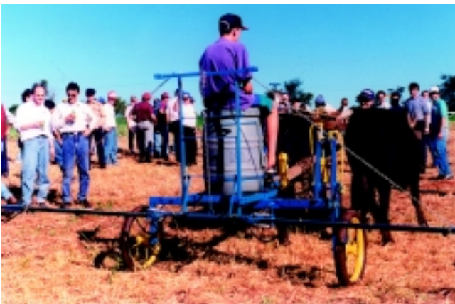
PLATE 91 Another version for animal traction with a round tank, 150 litres capacity, motor-cycle wheels, spray bar with 14 nozzles, and operator seat
