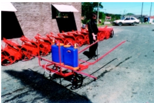
PLATE 85 Modification of two knapsack sprayers for animal traction, produced in the Itaiópolis municipality, Northern Santa Catarina
