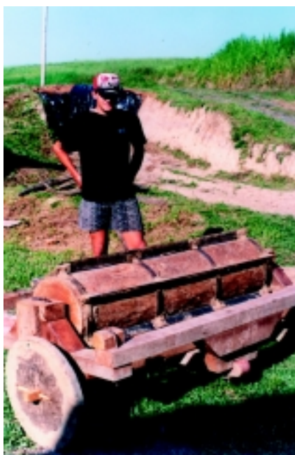
PLATE 78 Roller with blades manufactured by a farmer following an information folder from the Rural Extension Service, Dona Emma municipality, Alto Vale de Itajaí
