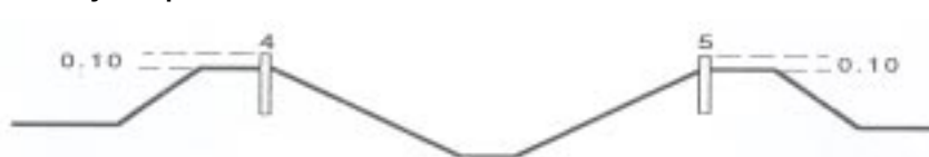
FIGURE A2.9-C Excavation nearly completed
