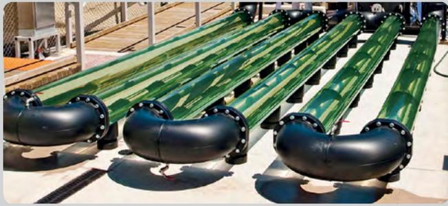
Spirulina can also be grown in Photo Bio-Reactors (PBR) or man-made machines specifically built to grow micro-algae; the fully controlled environment of the PBRs ensures a higher quality product with less waste and higher nutritional value. However the downside is that these machines are very expensive to buy and generally require specialised staff to operate them.
