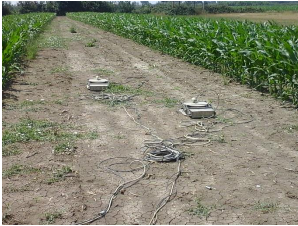
Figure 1. GHG field sampling system
