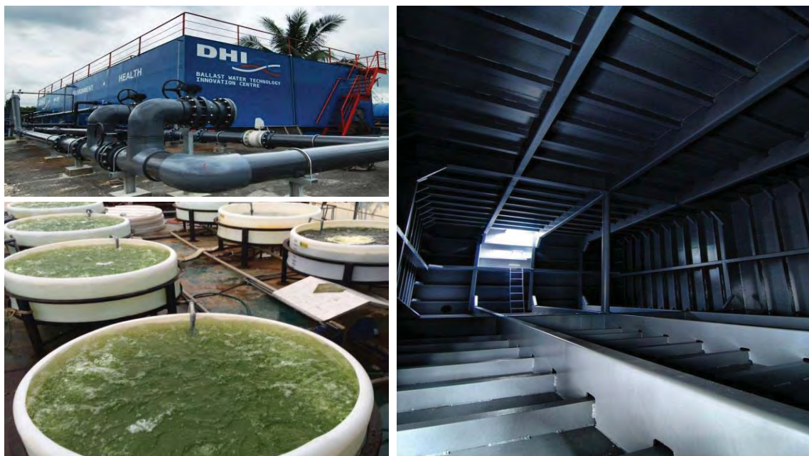
Fig. 3. Top left: the DHI ballast water technology and innovation centre in Singapore, bottom left: cultures of standard test organisms ( Tetraselmis sp.); right: inside a 250 m 3 retention tank used for mimicking ballast water transported during a ship's voyage.
