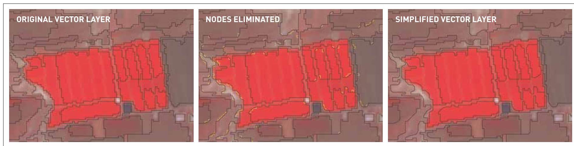
Figure 5. Detail of vector simplification. In yellow the nodes cut off in the procedure.
