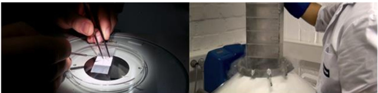
Left: Preparation of banana samples for cryopreservation. Right: Banana samples are plunged in liquid nitrogen at the International Transit Centre in Leuven. Credit: Bioversity International/N.Capozio
