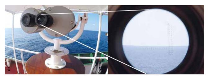
**Figure 5:** Bigeye binoculars (25 x 150): the angle ring and the reticule scale in the right ocular allow determining the angle and radial distance of the detection in relation to the ship.
