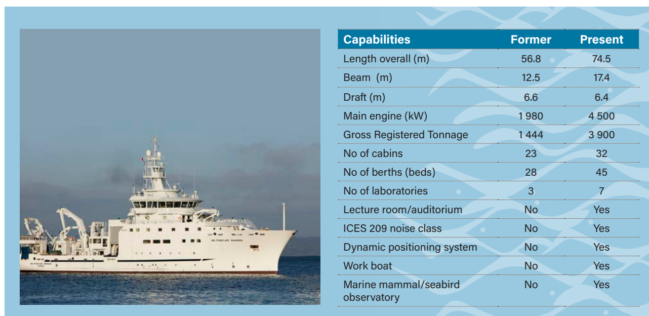
FIGURE 7. Main features of the new Dr Fridtjof Nansen and comparison with the former vessel.
