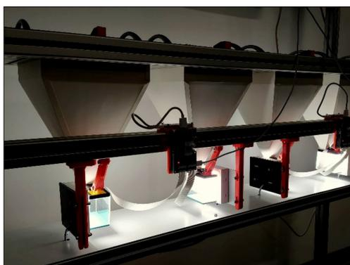
Fig. 2: Berlese Funnel equipped with sensor
