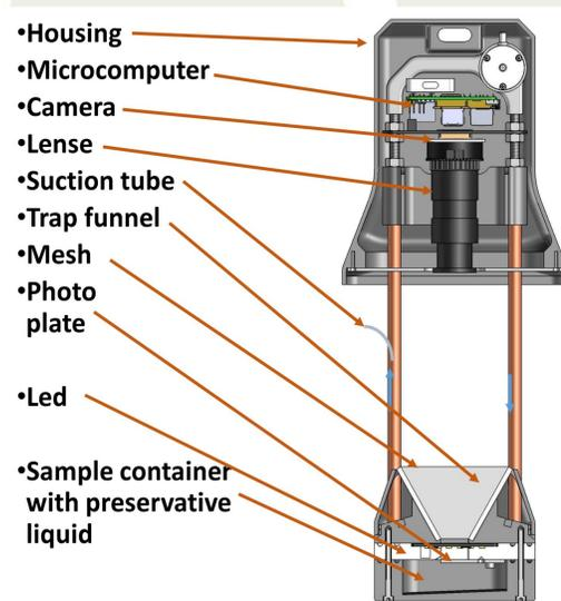
Fig.3: Cross sectional view of Edaphocam – model 2020
