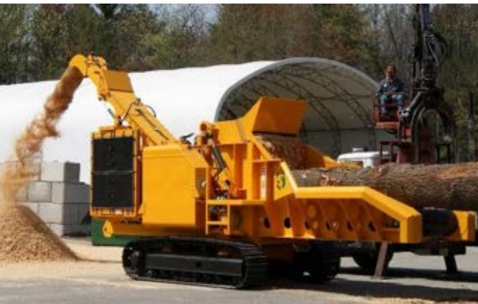
Figure 31 and 32: Large drum chipper processing stems with bark on and small drum chipper for smaller material
