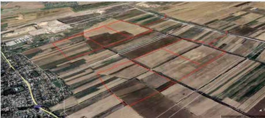
Concept for pump-buried pipe systems, each 90–100 ha, pumping from Secondary canal 4R2, Kzylkum Scheme
