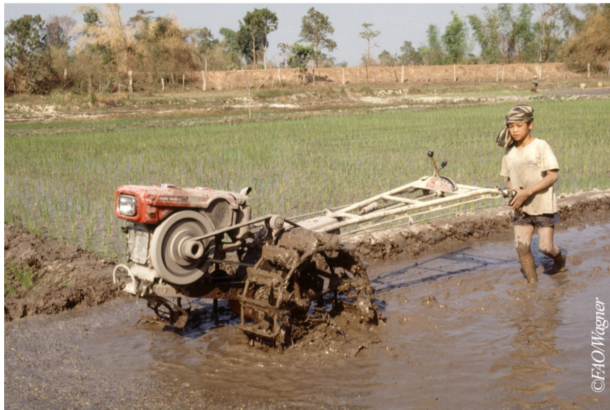
Preparation of a rice field using a mechanical plough.
