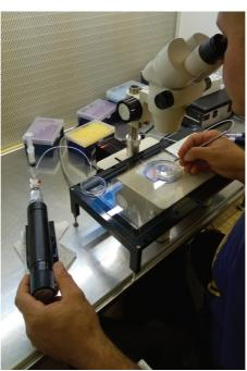
FIGURE A6.3.4 Fluid aspiration under stereomicroscope
