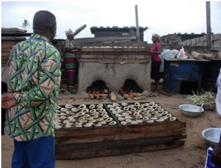
FIGURE 60 CHORKOR OVENS HAVE PROVED TO BE A POPULAR IMPROVED SMOKING KILN
