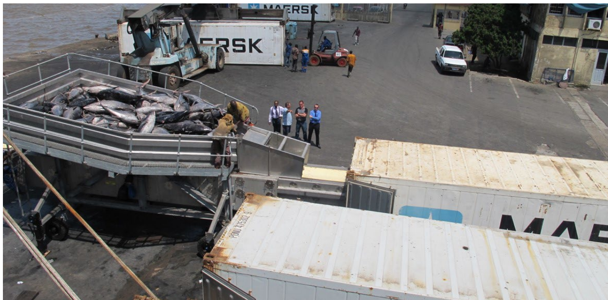
FIGURE 23: EXAMPLE OF IMPROVED EQUIPMENT FOR STUFFING CONTAINERS WITH TUNA
