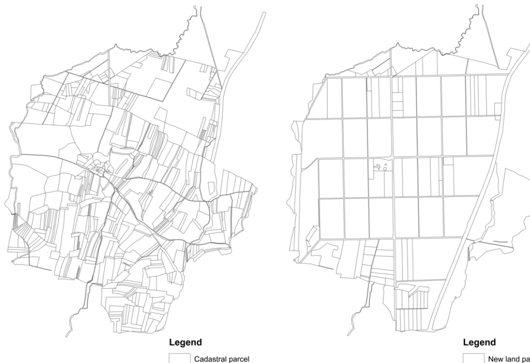
Dabjani land consolidation area - before land consolidation Dabjani land consolidation area - after land consolidation
