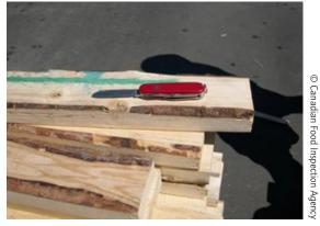
Board with knife on it is compliant because the knife is 2 cm by 15 cm and so the bark on the edge of the board is within tolerances; the board below it only contains discoloured cambium (no bark) and is therefore also compliant
