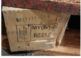
Mark is damaged and not legible
