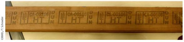
Mark matching example 1 of Annex 2 of ISPM 15 has additional information adjacent to the mark to indicate that the material is certified for use as dunnage
