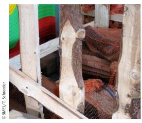
Bark exceeds tolerances: this wooden crate does not comply with ISPM 15
