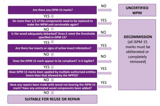
*Notes:* The flowchart provides examples of the types of questions that an authorized entity may use to evaluate a wood packaging unit in order to determine whether it is suitable for reuse or repair, or whether it should be decommissioned. Decommissioned wood packaging material units may be treated and recertified or they may be remanufactured, provided any remaining bark does not exceed the thresholds specified in ISPM 15.
