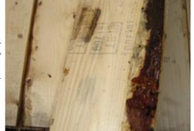
Bark on edge of board is less than 3 cm wide and therefore the board complies with bark tolerances
