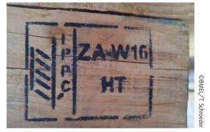
Mark, applied by stencilling, matches example 4 of Annex 2 of ISPM 15, with small gaps in the border and the vertical line
