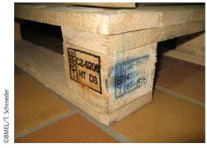
Two different ISPM 15 marks on one pallet block
