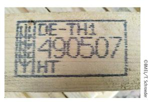
Mark, applied by an inkjet printer, is similar to example 2 of Annex 2 of ISPM 15 but producer/treatment-provider code is split over first and second line
