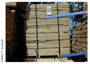
Dunnage that is integrated into packs of wood, such as the spacers or blocks indicated by arrows in this photograph, is not wood packaging material and does not need to be individually marked
