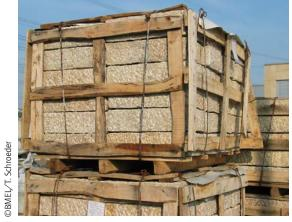
Wooden cage used to secure granite stones
