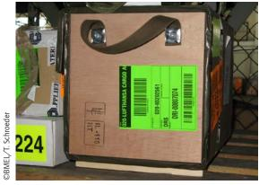
Composite box made from solid and processed wood
