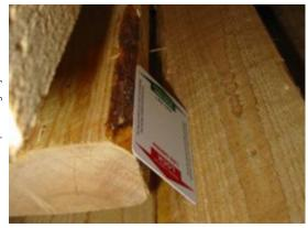
Bark on the edge of the wood is wider than 3 cm and the piece is greater than 50 cm<sup>2</sup>: the bark must be removed, or the piece may not be used for dunnage or to construct wood packaging material
